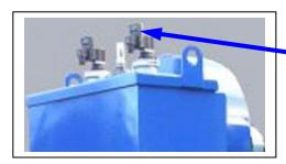
Each valve is fitted with an individual timer. The timer has two adjustable controls. The duration control marked "ms" should always be set to 100. The other marked "min" is the time between pulses and may be set to suit conditions, but not less than 0.5 minutes.
