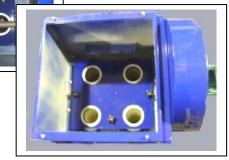
Unscrew and remove the knobs and washers from the cartridge clamping plates. Remove the clamping plates.
