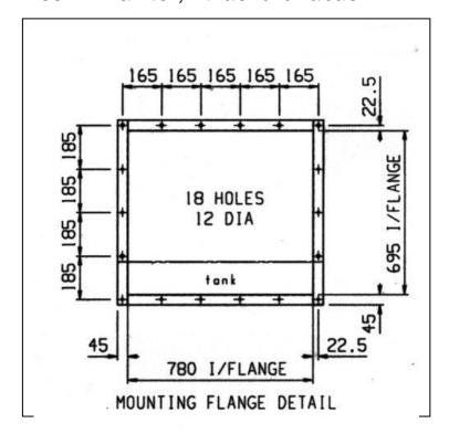
A suitable gasket or tube sealant material should be applied inboard of the base flange holes before bolting in place, to prevent leakage during normal use.
