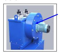
Remove the nuts securing the motor mounting plate to the fan case.
