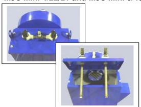
Remove the nuts securing the lid and lift off the lid, putting it in a safe position, so that the wiring and compressed air hose are not stressed.
