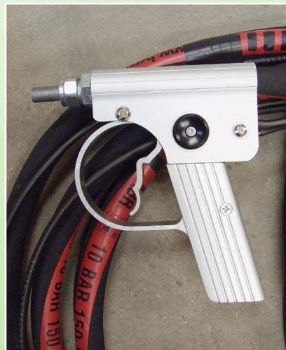
There is a combined air filter and pressure regulator and the standard blast nozzle is made of tungsten carbide. A vast range of nozzles can be used and the Ibimar operates with any type of inert material:
