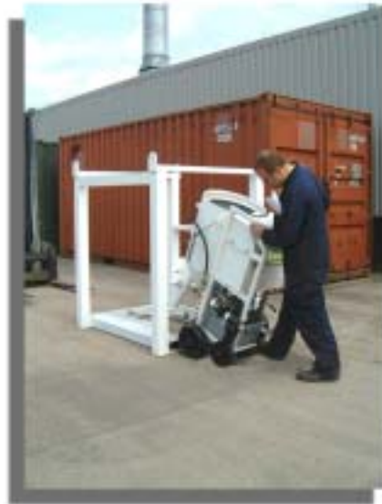
The machine can be removed from the frame giving greater manoeuvrability
